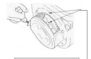
Align the mark on the starter pulley with the hole at the top of the recoil starter.
